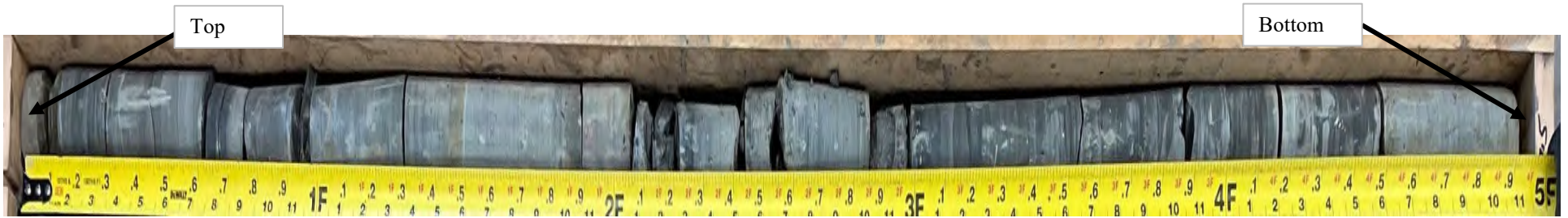
Photograph 1 Boring: B-1 Run 1 Depth 2.5'-7.5' See Photographs Nos. 2 and 3 for detailed views.
